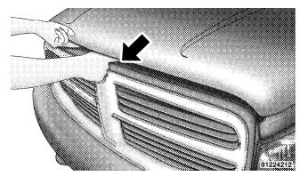
To prevent possible damage, do not slam the hood to close it. Use a firm downward push at the center of the hood to ensure that both latches engage. Never drive your vehicle unless the hood is fully closed, with both latches engaged.
